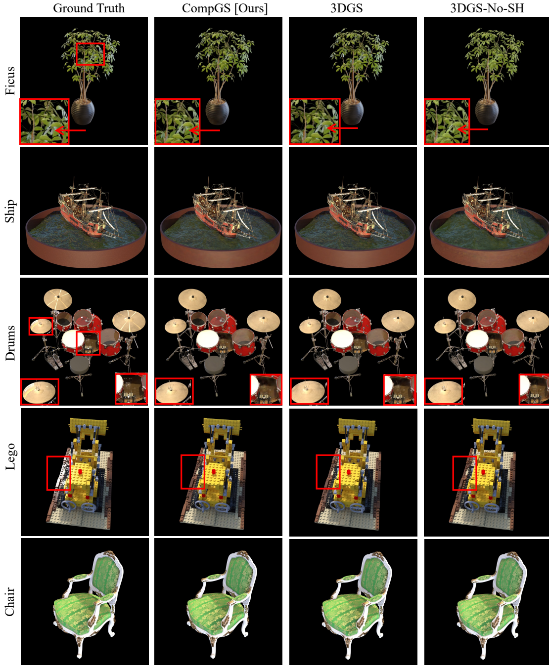
Figure 8. Visualization of results on Synthetic-NeRF dataset. We compare the performance of our compressed CompGS with the original 3DGS and 3DGS-No-SH approaches on different scenes of the NeRF-Synthetic dataset. The difference between CompGS and 3DGS-No-SH is apparent in some of these scenes. E.g., 3DGS-No-SH fails to effectively model the brown color of branches and shadows and bright light on the leaves of the ‘Ficus’ scene. All approaches including 3DGS have imperfect reconstruction in some of the scenes like ‘Drums’ and ‘Lego’. The scenes and views used for visualization were chosen at random.
